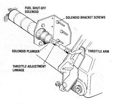
**NOTE:** The solenoid plunger **must** move smoothly and rapidly into the solenoid when the solenoid is electrically energized, drawing the engine's throttle arm into the Set Speed/Run Position.
