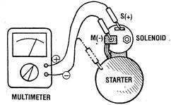
NOTE: Disconnect the wire from terminal M.
