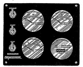
**PREHEAT:** The PREHEAT toggle switch serves two purposes: preheating the engine for easy starting and defeating of bypassing the engine oil pressure switch. The defeat function turns on the fuel solenoid, instrument power and alternator excitation.
