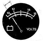
**NOTE:** When starting: A voltage drop will occur when the preheat switch is depressed.
