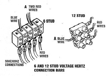
**NOTE:** When the optional voltage regulator is installed and if the Blue/White (Blue) lead is not correctly positioned to correspond to the Hertz the unit is operating at, the regulator will sense incorrect voltage and cause the generator to produce abnormally high output voltage.
