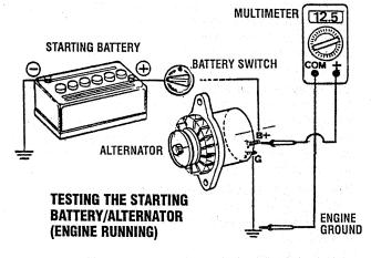
8. Start the engine again. Check the voltage between the alternator output and ground.
