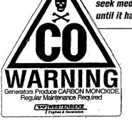
A WARNING DECAL is provided by WESTERBEKE and should be fixed to a bulkhead near your engine or generator.
