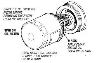
2. Replacing the Oil Filter. When removing the used oil filter, you may find it helpful and cleaner to punch a hole in the upper and lower portion of the old filter to drain the oil from it into a container before removing it. This helps to lessen spillage. A small automotive filter wrench should be helpful in removing the old oil filter.
