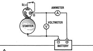
**CAUTION:** Use thick wires as much as possible and tighten every terminal securely. This is a solenoid shift-type starter which makes a rotating sound louder than that of a direct-drive type starter. When detecting starter rotation at the pinion tip, be careful not to come in contact with the pinion gear when it protrudes.
