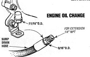
1. Draining the Oil Sump. Discharge the used oil through the sump drain hose (attached to the front of the engine) while the engine is warm. Drain the used oil completely, replace the hose in its bracket, and replace the end cap securely.
