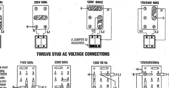
The frame ground wire must be moved when changing from 115 volts and 110/220 volts 50 hertz to 230 volts 50 hertz. From making connections to the AC terminal block, use terminal ends for 1/4 inch studs that will accept multi-strand copper wire sized for the amperage rating from the hot lead connection. The frame ground wire is white or white with a green strip. It connects between the neutral stud and the generator frame.
